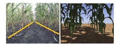
Fig. 5. Real and simulated camera images for corn row following for agricultural robots.
